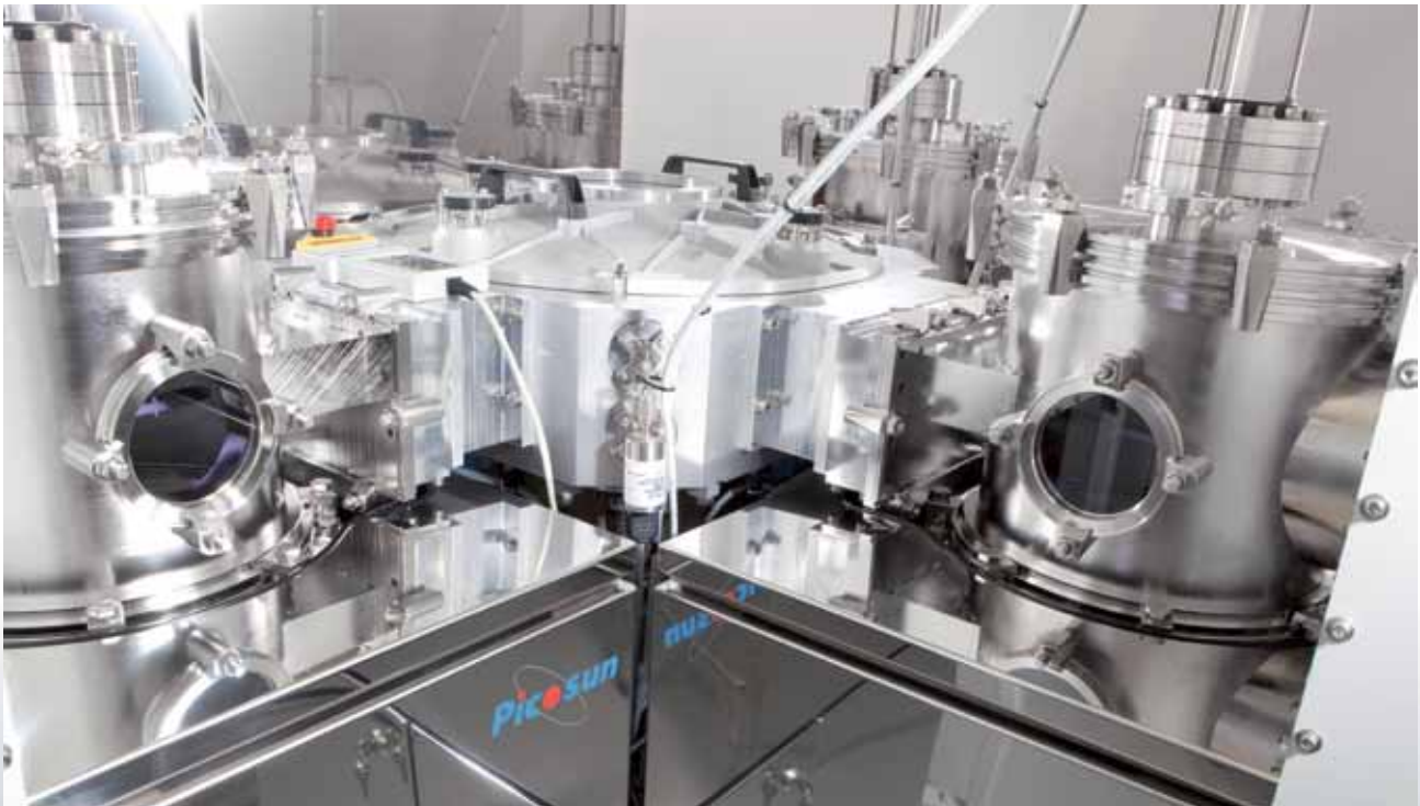
PICOPLATFORM™ 200 ALD cluster tool with four PICOSUN™ R-series ALD reactors.
