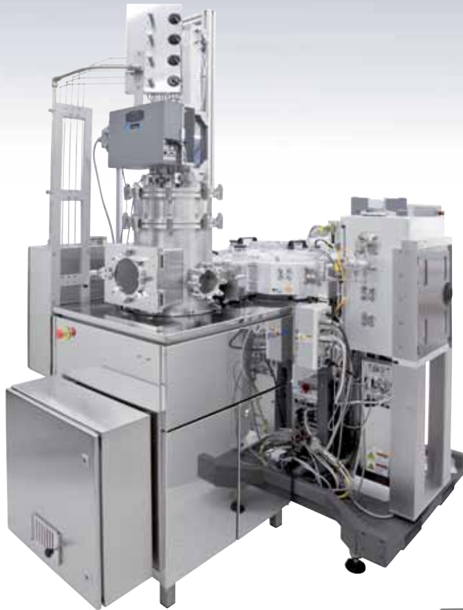
PICOSUN™ R-200 Advanced ALD tool with a plasma generator integrated into a PICOPLATFORM™ 200 cassette-to-cassette loading cluster system.
