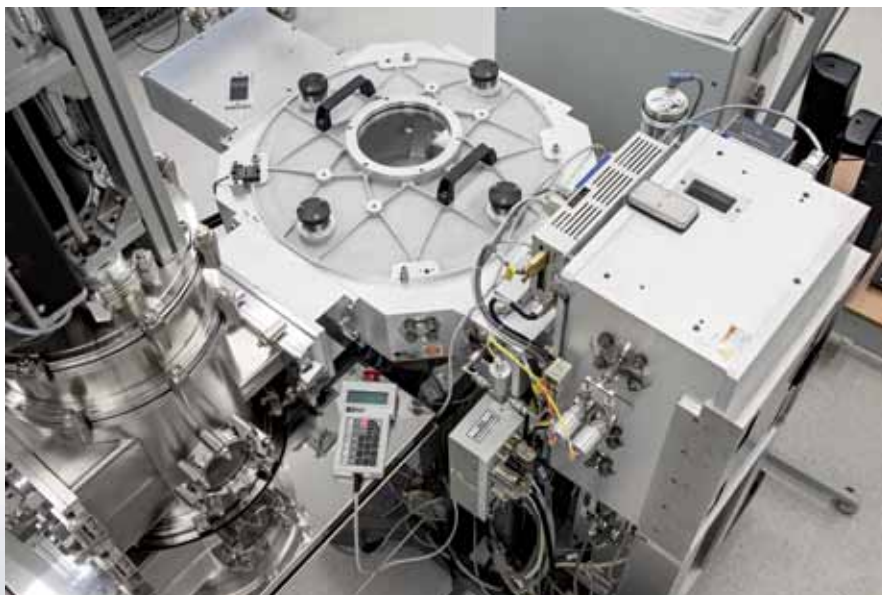
PICOPLATFORM™ 200 ALD cluster tool with an automatic cassette-to-cassette loader.
