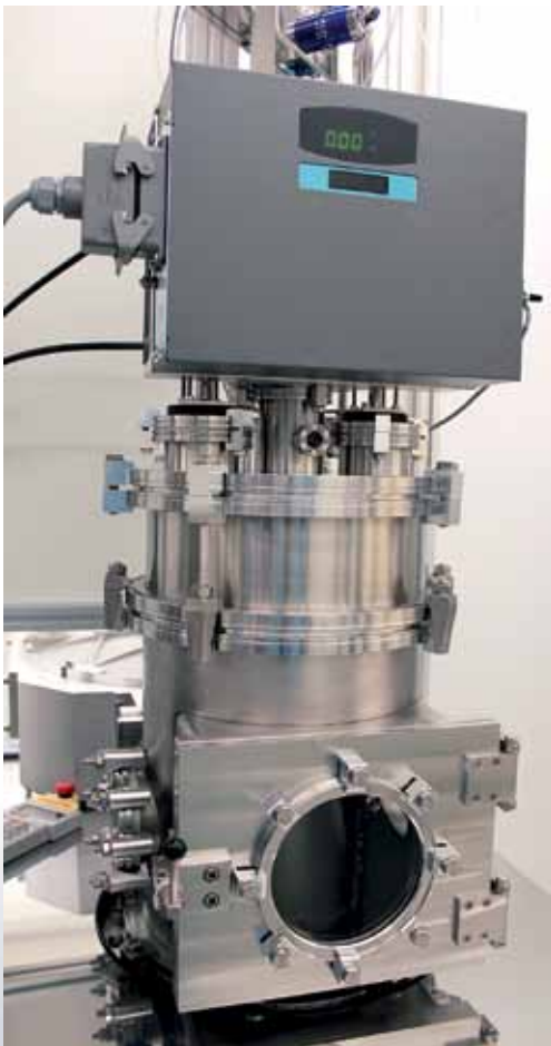
PICOPLASMA™ source system installed on a PICOPLASMA™ R-series ALD reactor.
